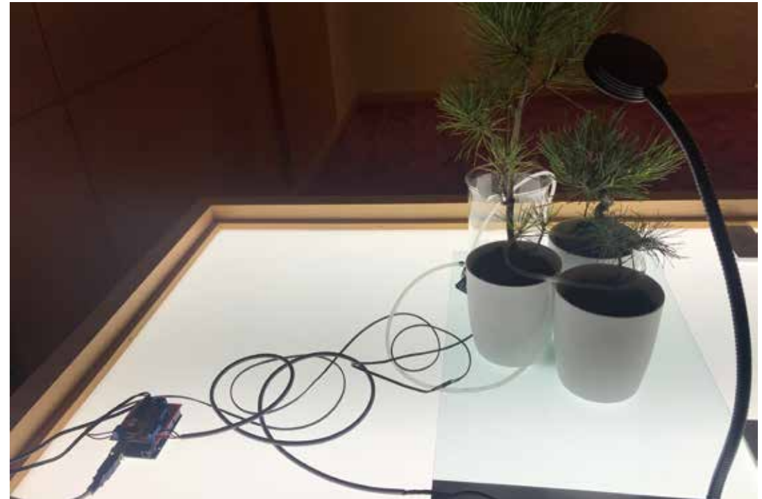
When lightning strikes, water is given through the tube, and after a certain number of lightning strikes LEDs for plant growth change from red to blue to purple to encourage growth and nurturing.
